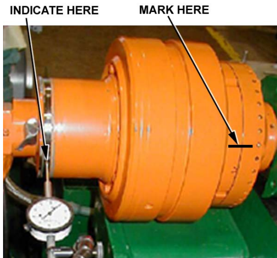
PLUNGER POSITIONED AT HORIZONTAL CENTERLINE OF ROTODIFF
