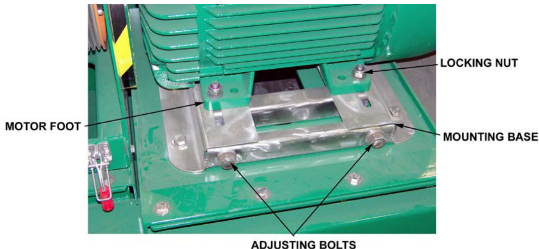
Figure 4-2 Drive Belt Tension Adjustment
