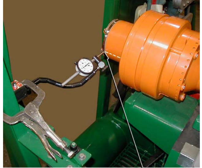
PLUNGER POSITIONED AT HORIZONTAL CENTERLINE OF GEARBOX
