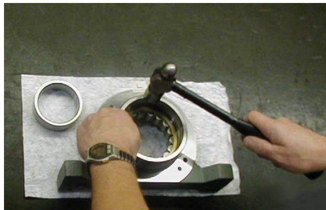
TAPPING BEARING INTO PILLOW BLOCK
