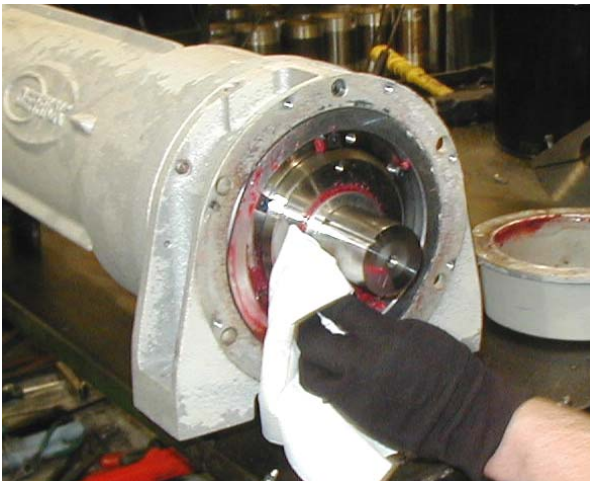
5 - Using a soft absorbent cloth, remove excess lubricant from components. Do not use compressed air for cleaning as this may drive contaminants into motor.
