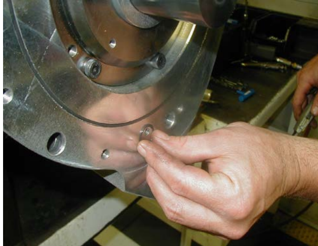
10 - Lightly lubricate and install both main cover O-ring and oil drain O-ring.
