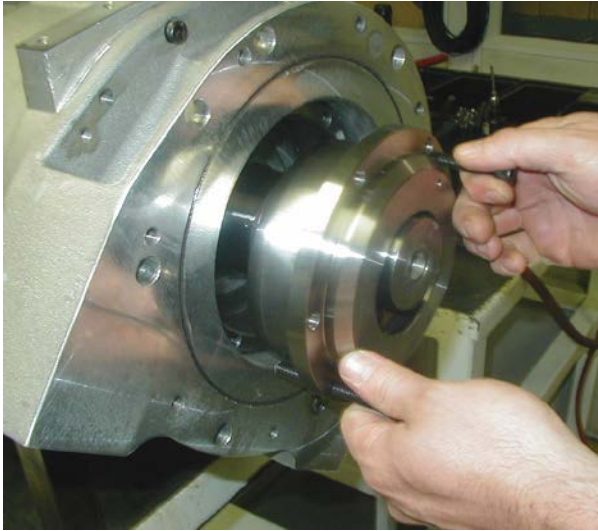
14 - Remove and discard bearing and bearing mount.
