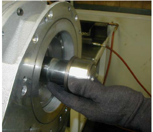
17 - Carefully remove and discard heated inner bearing race from motor shaft. Using a soft absorbent cloth, remove excess lubricant from interior of bearing housing.
