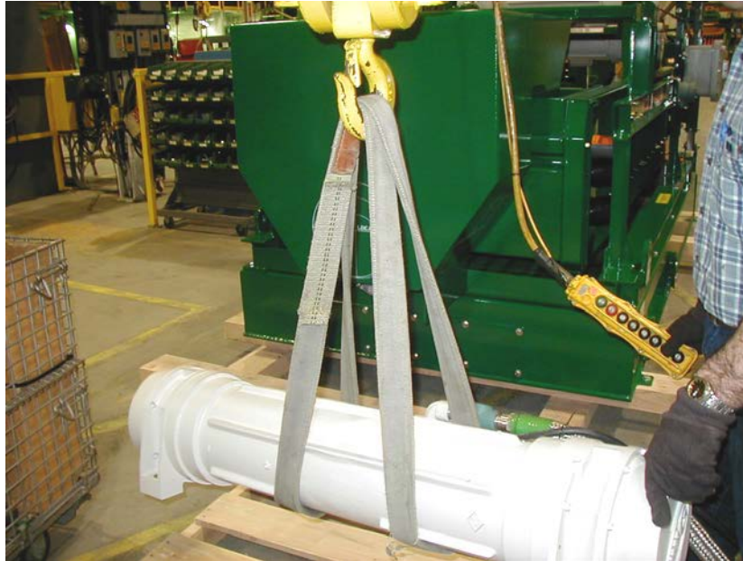
Figure 1. Hoisting Sling Position
