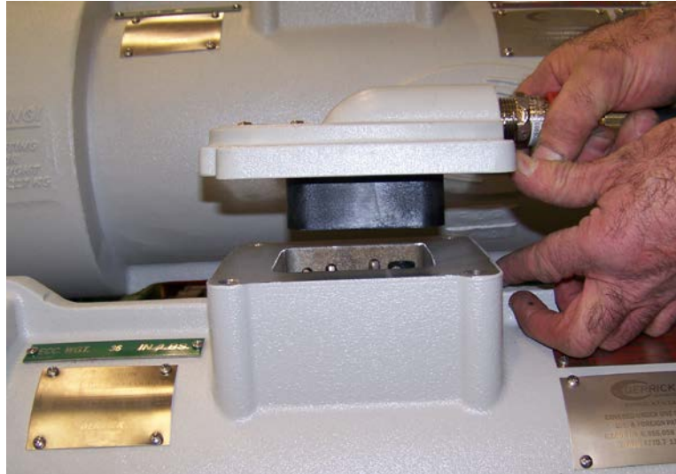
Figure 4. Mating Power Connector with Motor Junction Box
