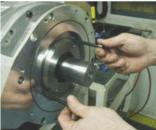
12 - Carefully thread jack bolts into threaded holes in bearing mount, being sure to avoid cross-threading.
