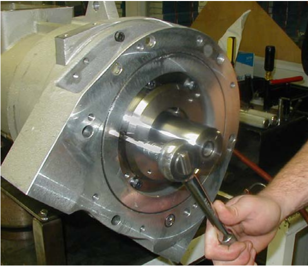
10 - Using a 6mm hex wrench, remove six M8 screws securing bearing mount to bearing housing.
